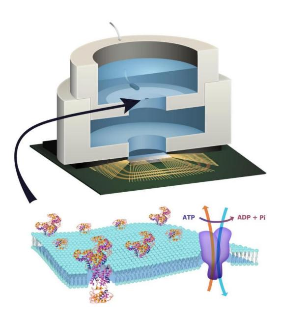
Biocell attached to CMOS integrated circuit with membrane containing sodiumpotassium pumps in pore. Credit: Trevor Finney and Jared Roseman/Columbia Engineering
