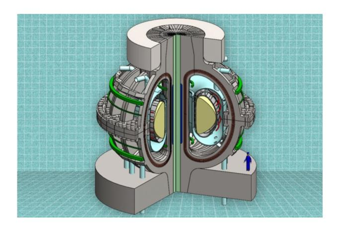
A cutaway view of the proposed ARC reactor. Thanks to powerful new magnet technology, the much smaller, less-expensive ARC reactor would deliver the same power output as a much larger reactor. Credit: the MIT ARC team
