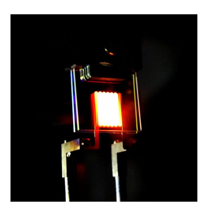
A nanophotonic incandescent light bulb demonstrates the ability to tailor light radiated by a hot object. Credit: MIT
