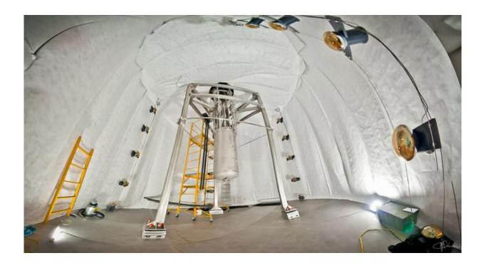
The LUX Dark Matter Experiment operates a mile underground at the Sanford Underground Research Facility. It's location helps shield the detector from background radiation that could confound a dark matter signal. Credit: C. H. Faham
