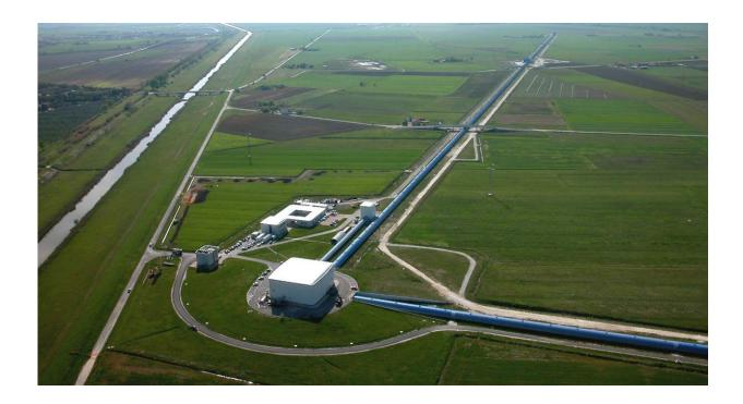
Aerial view of the Virgo site showing the Mode-Cleaner building, the Central building, the three kilometer-long west arm and the beginning of the north arm. The other buildings include offices, workshops, computer rooms and the control room of the interferometer. Credit: The Virgo collaboration/CCO 1.0
