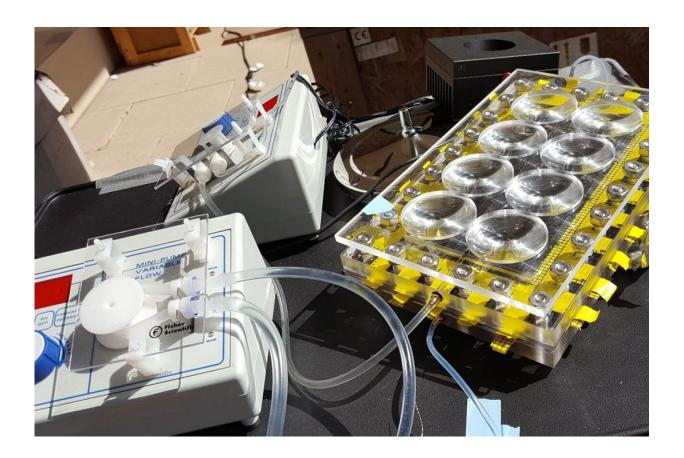
Researchers from Rice University's Laboratory for Nanophotonics found they could boost the efficiency of their solar-powered desalination system by more than 50% by adding inexpensive plastic lenses to concentrate sunlight into "hot spots." . Credit: Pratiksha Dongare/Rice University
