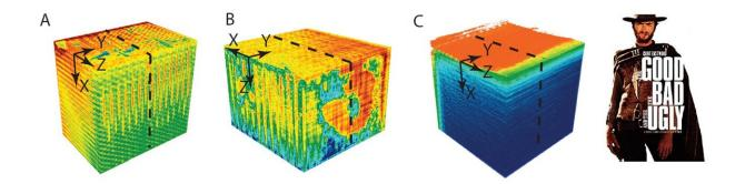
Figure 3. Birds-eye view of reconstructed 3D silicon nanostructures shown in the SEM images in Fig. 1. (A) 3D photonic crystal that reveals a broad photonic gap in agreement with theory: "the Good". (B) 3D photonic crystal that reveals a large void due to stiction resulting from violent liquid evaporation in the pores:
