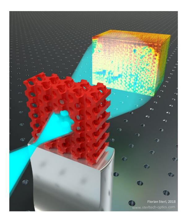
Figure 2. Animation sequence showing that TXT data are recorded while rotating the sample (three orientations are shown). From the recorded radiographs, the tomographic reconstruction is derived that is shown in the background. Credit: Diana Grishina
