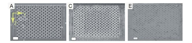
Figure 1. Electron microscope images of three 3D photonic crystal nanostructures fabricated in the same way. Each external surface looks closely matches the design and looks like the other, but the functionality and internal structure will appear to be completely different. Credit: Diana Grishina
