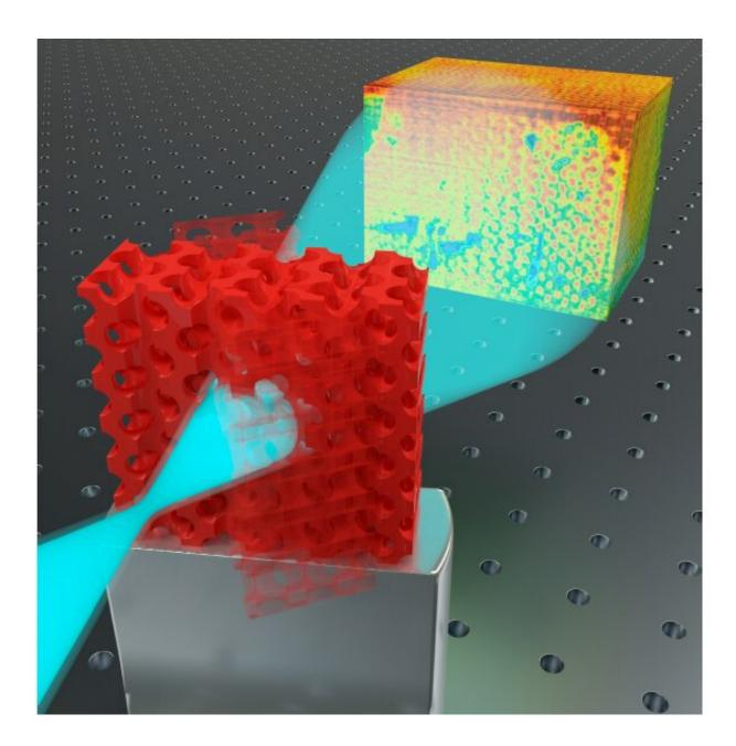
Figure 2. Animation sequence showing that TXT data are recorded while rotating the sample (three orientations are shown). From the recorded radiographs, the tomographic reconstruction is derived that is shown in the background. Credit: Diana Grishina
