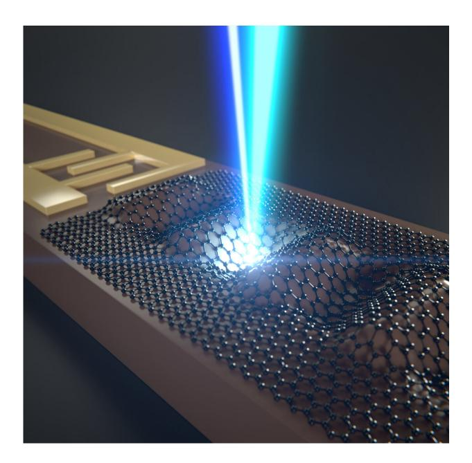
A surface acoustic wave generated with an interdigital transducer deforms the graphene inducing strain in the lattice and modifying its phonons, and thus the Raman response of the material. Credit: Jorge Pedrós, Rajveer Fandan (UPM) and Enrique Sahagún (Scixel).
