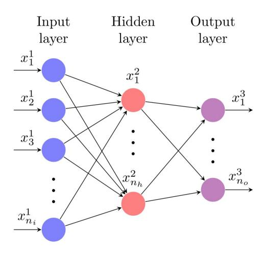
Schematic of a plain neural network. There are three layers, with input on left through output on the right. Each circle represents a node. Credit: Santak, P., & Conduit, G. (2019). Predicting physical properties of alkanes with neural networks. Fluid Phase Equilibria, 401, 112259. DOI: 10.1016/j.fluid.2019.112259
