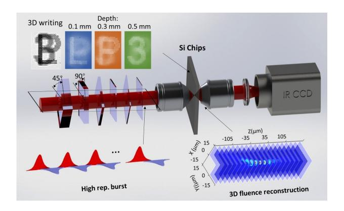
Researchers demonstrate multi-layer writing deep inside silicon by using tightly focused ultrashort pulses at THz-repetition-rate. Credit: LP3-CNRS.
