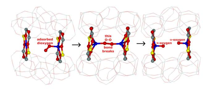
Simplified reaction scheme of the formation of the Alpha-oxygen atoms from dioxygen over the ferrierite matrix with the distant binuclear iron centers. The iron atoms are in blue, oxygen in red, silicon in gray, and aluminum in yellow. The atoms of the cationic sites are depicted as balls. Credit: Stepan Sklenak
