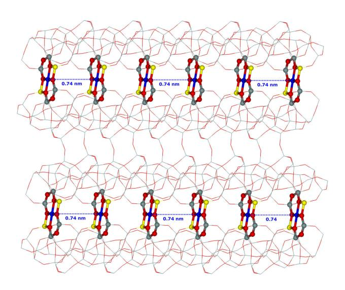
The simplified structure of the ferrierite matrix with the distant binuclear iron centers. The iron atoms are in blue, oxygen in red, silicon in gray, and aluminum in yellow. The ferrierite structure is periodic in all the three dimensions. The
