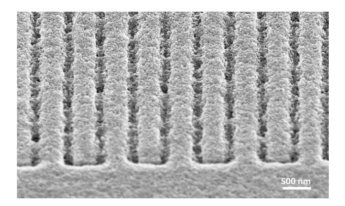
Oblique incidence scanning electron microscope image of a plasmonic electro-optic metasurface covered with barium titanate nanoparticles. Credit: Artemios Karvounis
