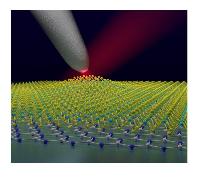
Schematic of a laser-illuminated nano-optical probe investigating a strained
