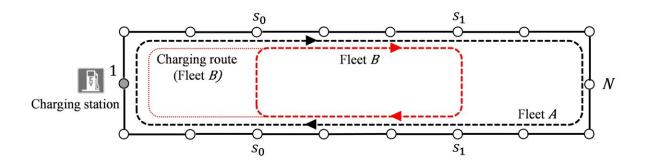
The bus operating the short turning line serves the passengers between stops s0 and s1, if the bus needs to recharge battery at the charging station, it will run without passengers as soon as possible from stop s0 to the charging station. After fully charging the battery, the bus will deadhead back to stop s0 and start the next service circulation. Credit: Dr. W. Zhang and Dr. M. Xu
