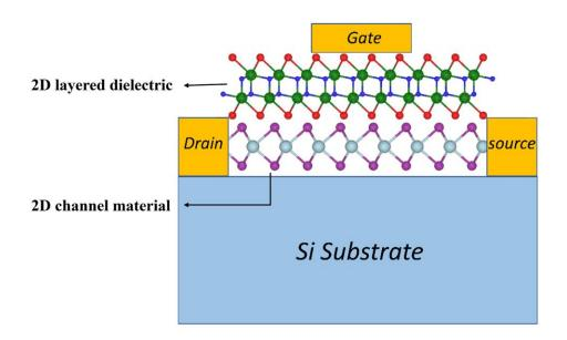
Figure 1: A simplistic schematic of an ultra-thin transistor made with a 2D layered dielectric and a 2D channel material. Credit: Mehrdad Rostami Osanloo, Author provided.
