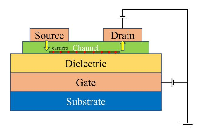
Figure 2: A simplistic view of a field-effect transistor. A good dielectric minimizes the excessive flow of current through the gate. Credit: Mehrdad Rostami Osanloo, Author provided.
