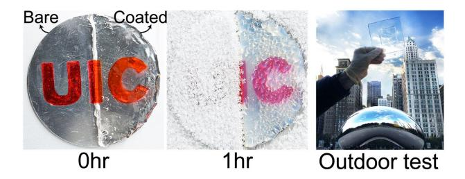
A metal disc half-coated with our anti-freezing gel remains optically transparent under frigid conditions (cooling temperature =-30°C and relative humidity=60%) while the bare section gets enveloped in a thick forest of frost. Rightmost image shows a gel-coated glass plate retaining its transparency without frosting in wintry outdoor conditions (air temperature = -2°C and relative humidity=70%) of Chicago, IL, USA (December 2020). Credit: Rukmava Chatterjee
