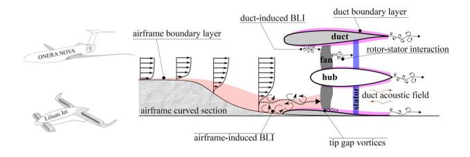
Complex noise sources illustration in an embedded engine or boundary layer ingesting (BLI) ducted fan. Credit: Feroz Ahmed
