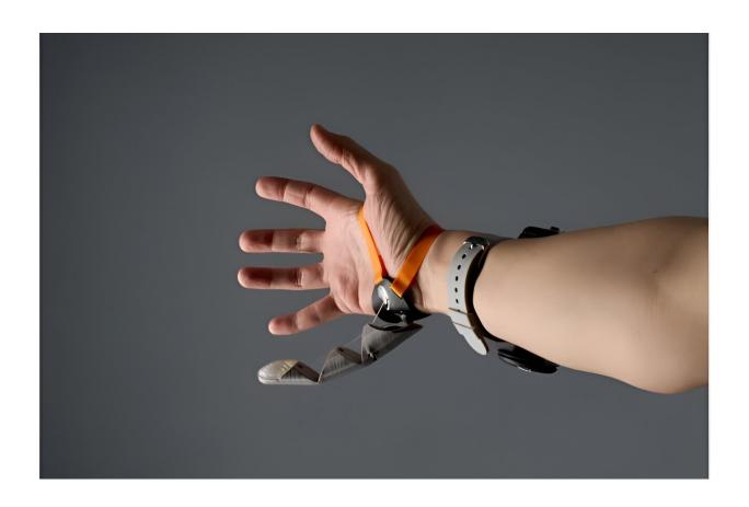
Image showing the Third Thumb design from the perspective of the wearer. Credit: Dani Clode Design & The Plasticity Lab
