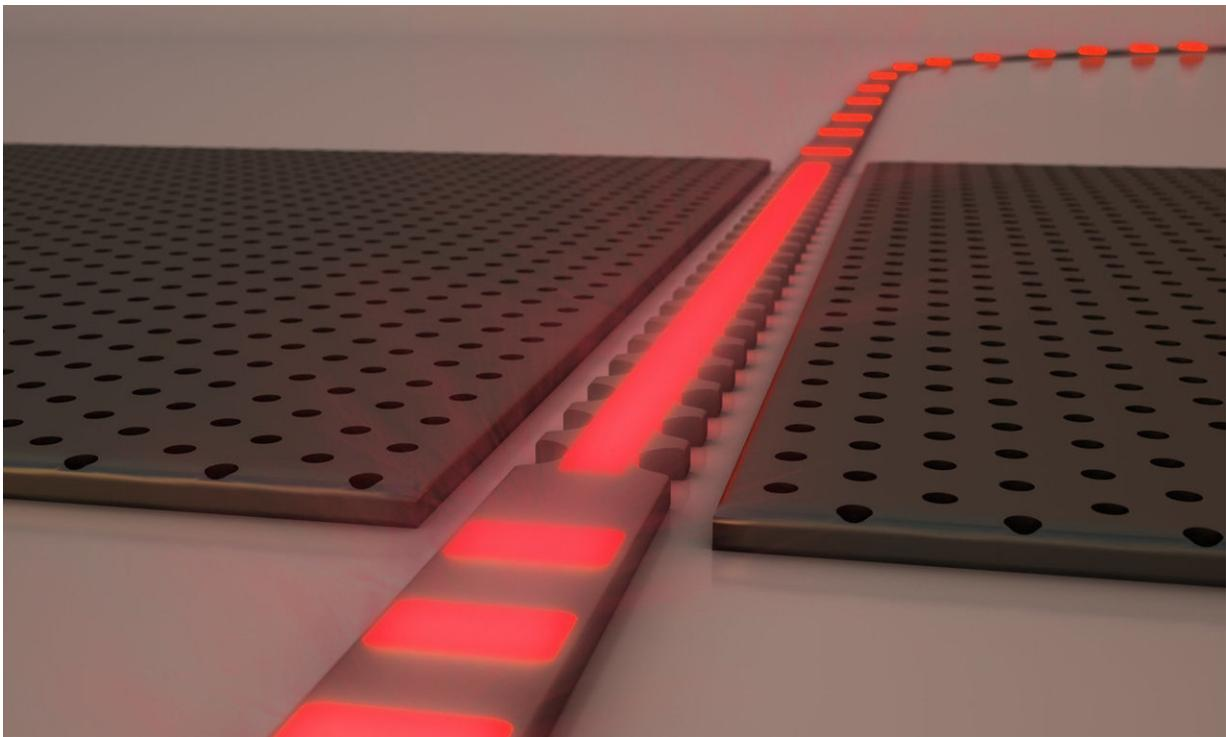
A zero-index waveguide compatible with current silicon photonic technologies.
