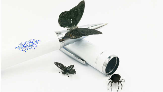
Mini kirigami SLiR thin-film robots. Credit: Ghim Wei Ho and Xiao-Qiao Wang
