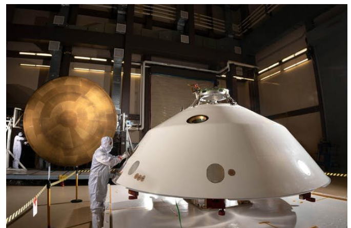
Pictured are the Mars 2020 backshell heat shield (foreground) and the main PICA heat shield (background). Credit: NASA/JPL-Caltech
